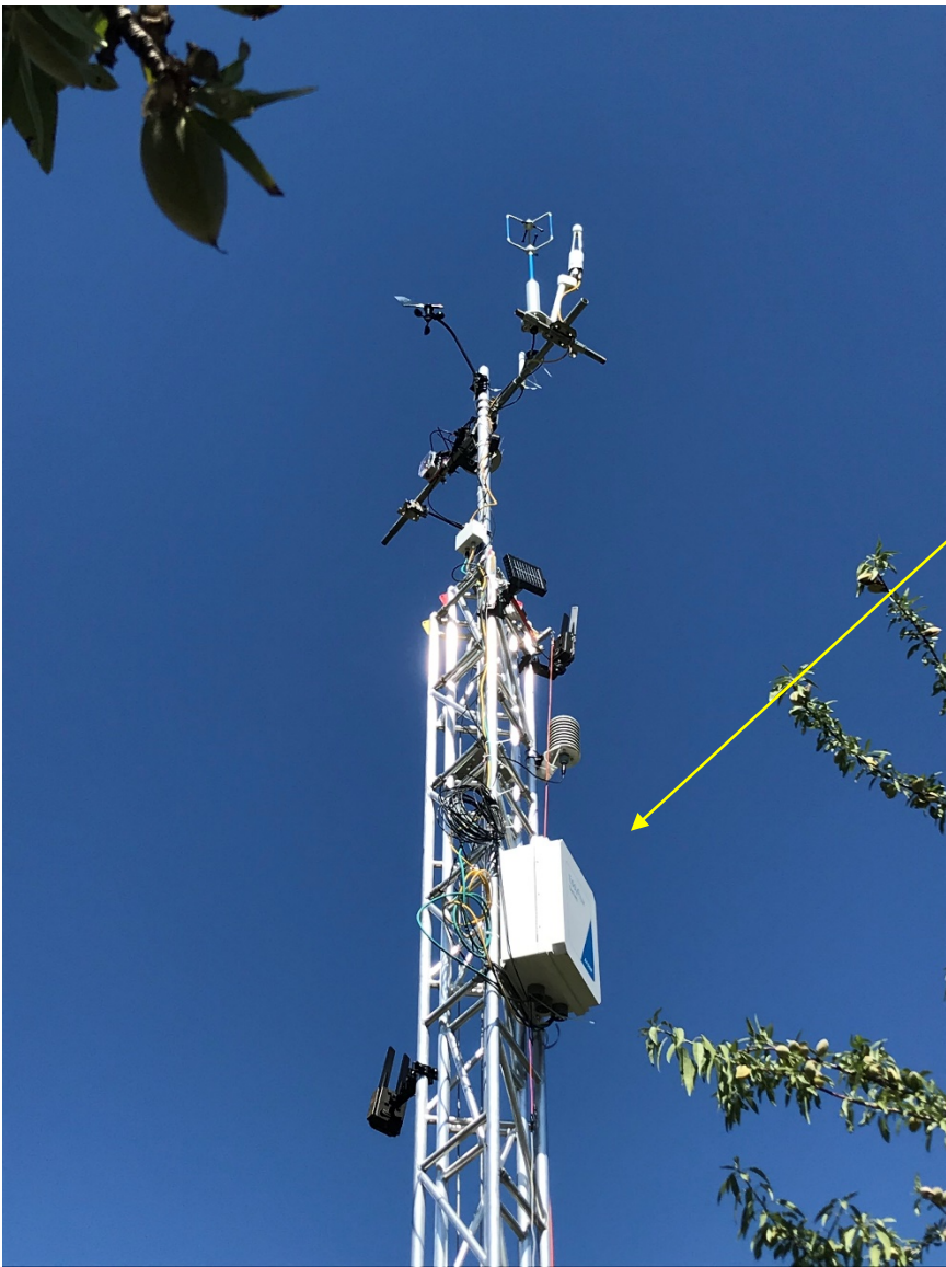
Eddy Covariance flux tower for validation of remote sensing ET
