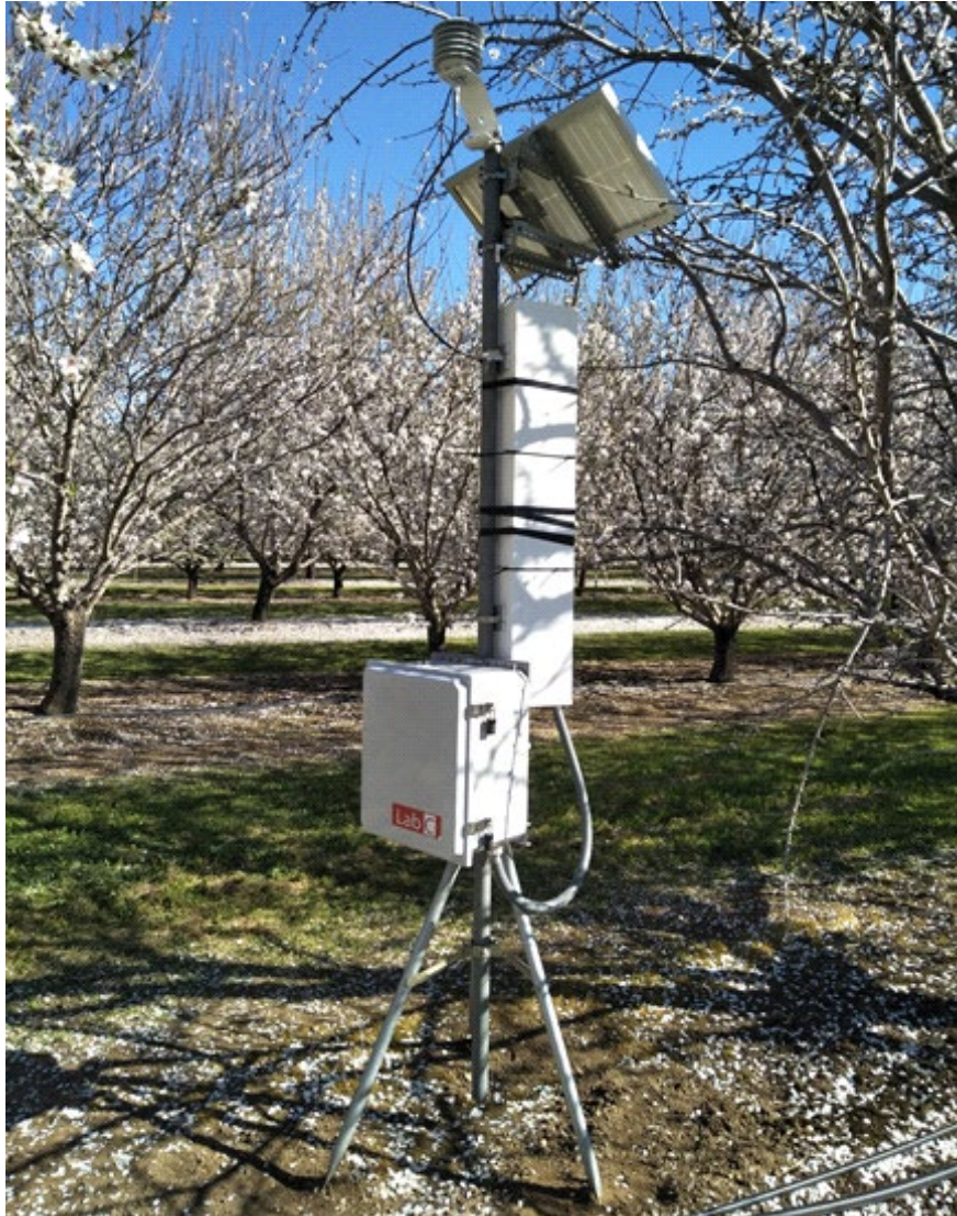
Large area cosmic ray soil moisture sensing
