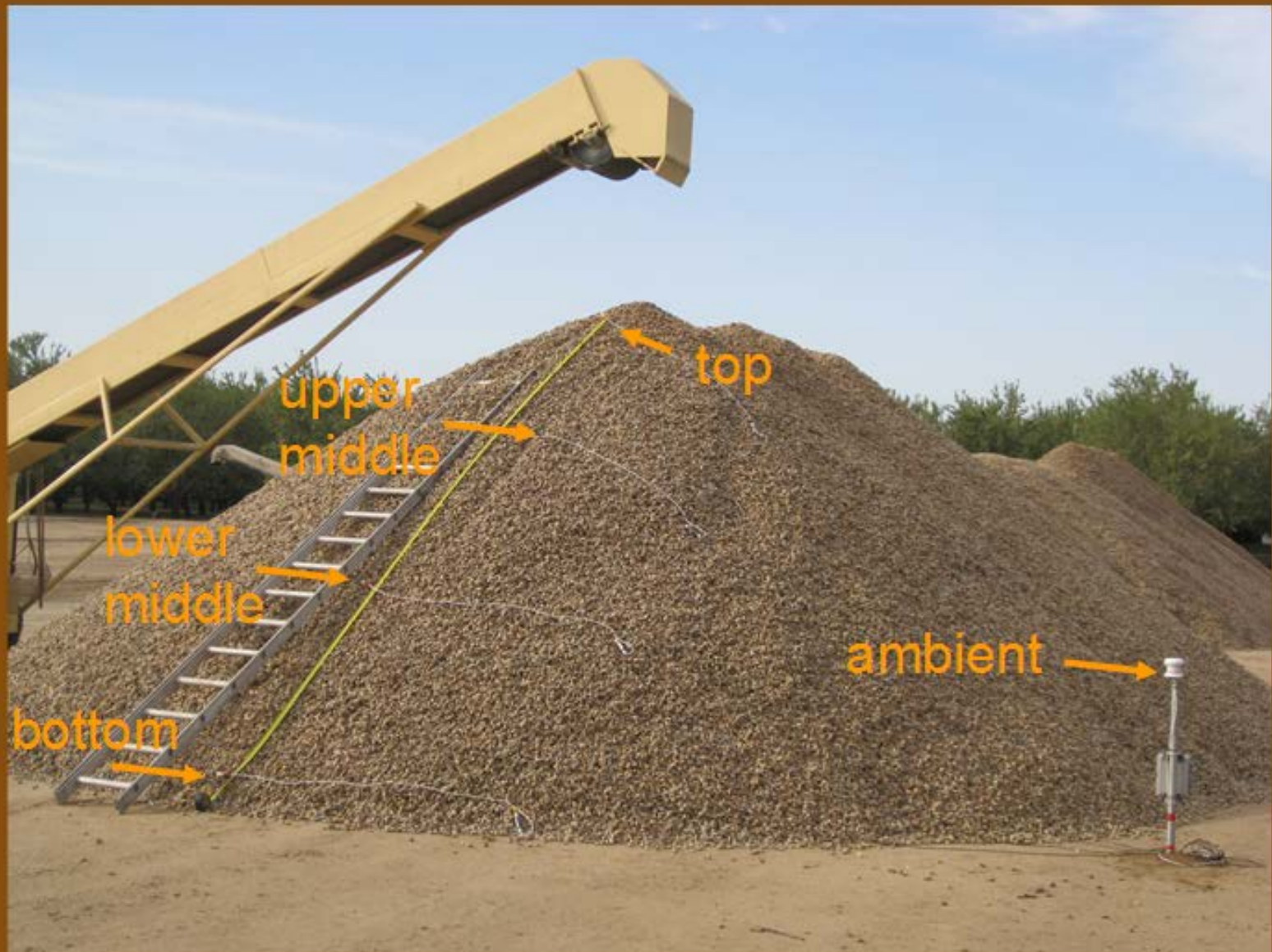
Temperature and relative humidity sensor placement in stockpiles. Sensors were approximately in the middle of the stockpiles long dimension in line with the yellow measuring tapes.
