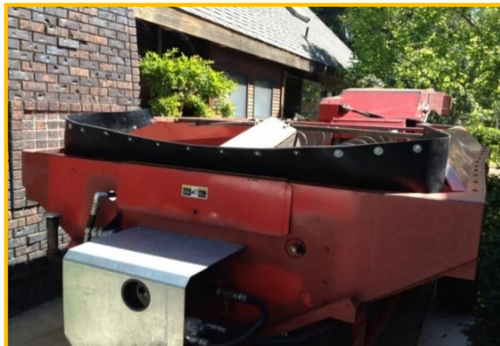
Front skirt to prevent nuts from overflowing as cart fills
