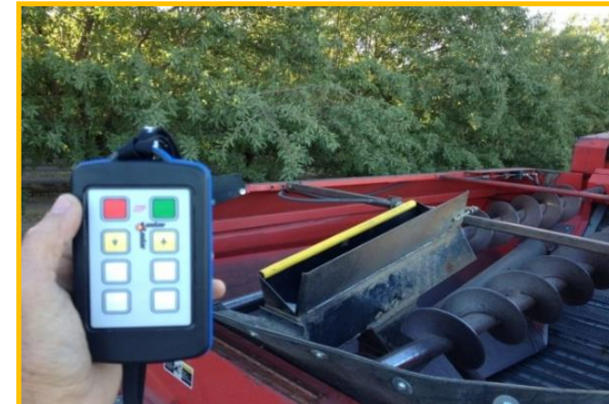
Wireless controller for hydraulically operated auto sampler
