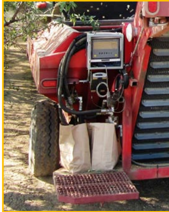
Trimble GPS acts as datalogger to collect continuous yield data
