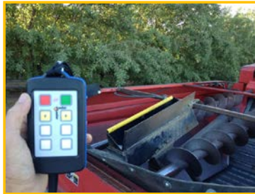
Wireless controller for hydraulically operated auto sampler
