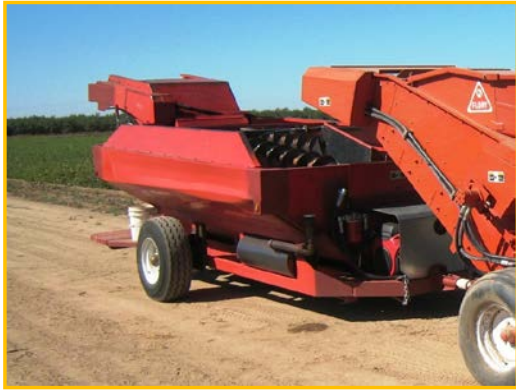
Self contained hydraulic system for operating augers, autosampler and elevator
