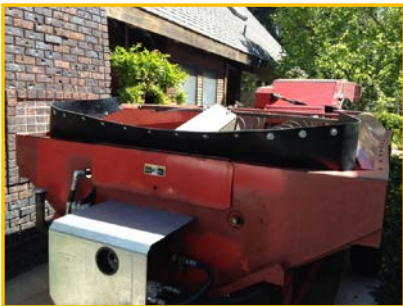
Front skirt to prevent nuts from overflowing as cart fills
