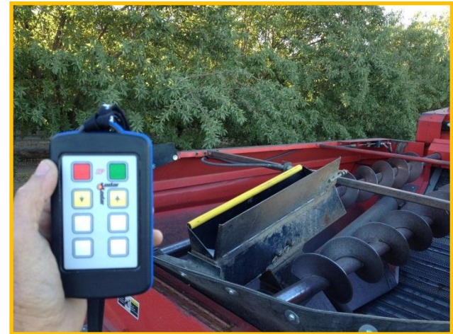
Wireless controller for hydraulically operated auto sampler
