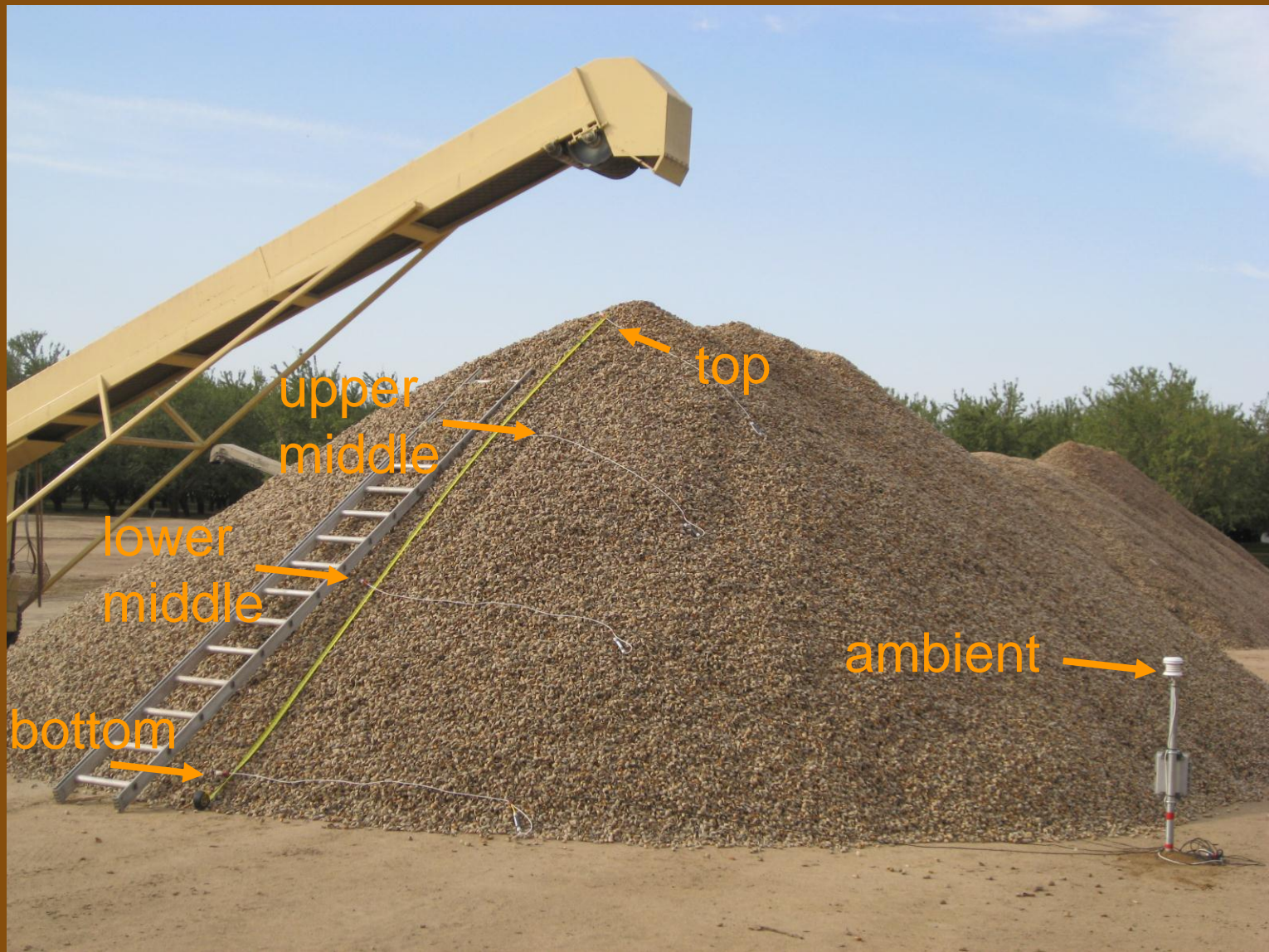
Temperature and relative humidity sensor placement in stockpiles
