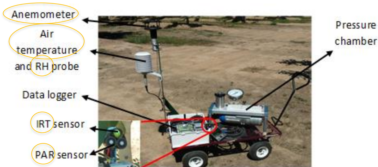
Figure 2. Mobile sensor suite and pressure chamber during data collection in an almond orchard.
