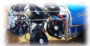
ZeferSpray PTO TRX cone jet Nozzles – 4/fan
