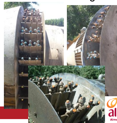
Air-O-Fan D-240 TRX cone jet nozzles Maximal configuration
