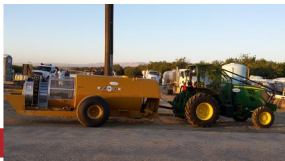
Air-O-Fan 232 PTO 1000 gal tank
