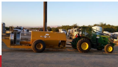
Air-O-Fan 232 PTO 1000 gal tank Hollow cone
