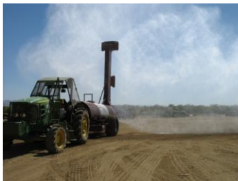
Progressive Ag Tower 150 gals/ac @ 3 mph
