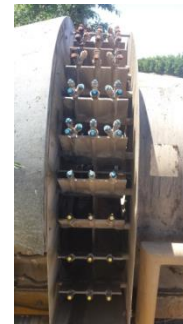
Air-O-Fan D-240 TRX cone jet nozzles Minimal configuration
