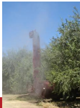
Progressive Ag Tower 150 gals/ac @ 3 mph
