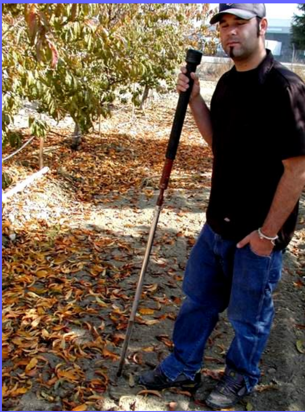
3 foot push or slide hammer probe ($150-$250)
