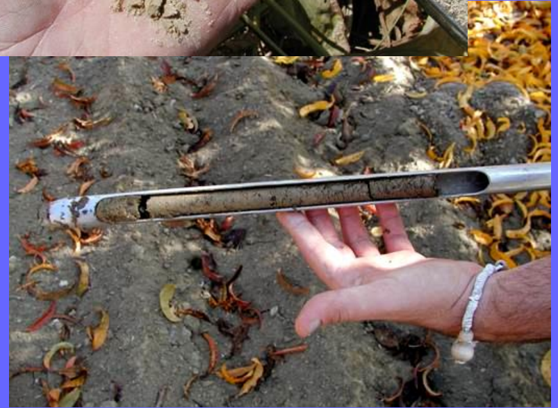
3 foot push or slide hammer probe ($150-$250)
